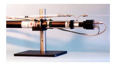
Detail of sensor head and supporting optical base. The sample is fed in through the 1/8 in diameter stinger tube (top right) and passes through the self-aligning optical system before exiting through the 1/4 in diameter exhaust tube, connected to the main control unit. All control electronics and instrumentation are contained in the main control unit for ease of operation and convenience.
